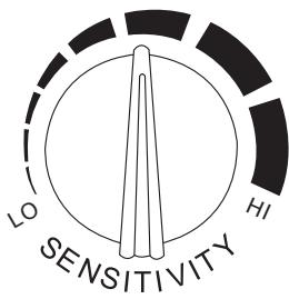
Before welding, please adjust the sensitivity to high position, if encountering the interference of Lighting lamp(the filter is darkening while not welding),please adjust the sensitivity towards low position slightly until the filter returns to light state (please don't make the helmet towards to light lamp source during this process, should towards to welding workpiece). During welding, the sensitivity knob should be adjusted as high as possible, or it will affect the darkening speed of filter.
